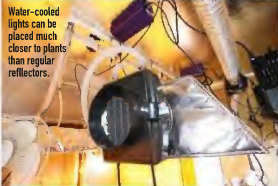
The reservoir keeps lights constantly cool.
